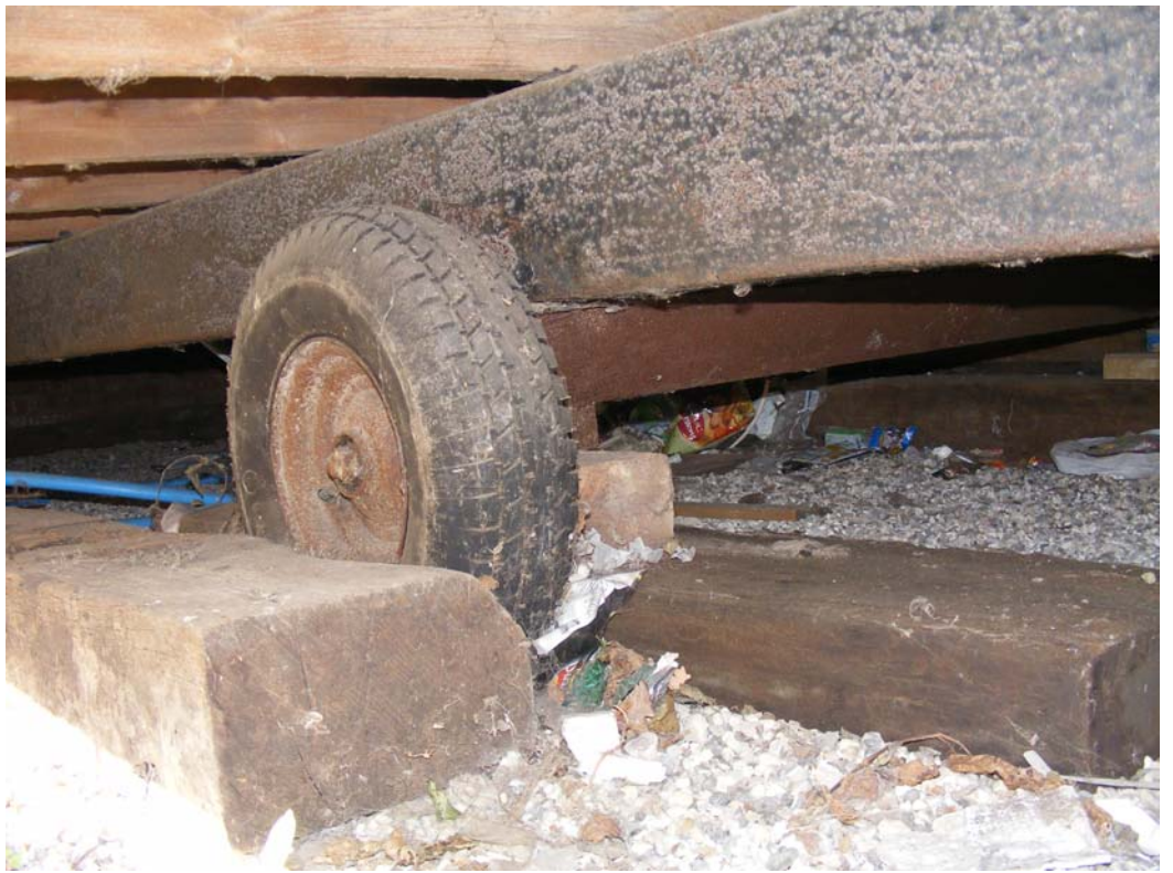
Typical Chassis with the delivery wheels lifted from the ground to spin freely
